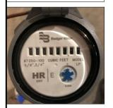
**Top/Register:** Device attached to the Base/Bottom which records water usage data. The Top/Register is either round with an odometer-like dial or a rectangle with a digital display.
